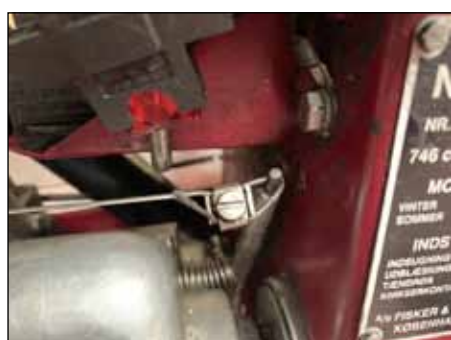
Where there's a will, there's a way (I) - like here where parts from a local bicycle shop was used for an emergency repair of the clutch cable.
