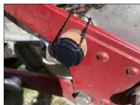
Where there's a will, there's a way (II) - like here where a bottle of Cava had to be downed, so its cork could be used to prevent dirt from entering the rear drive housing.
